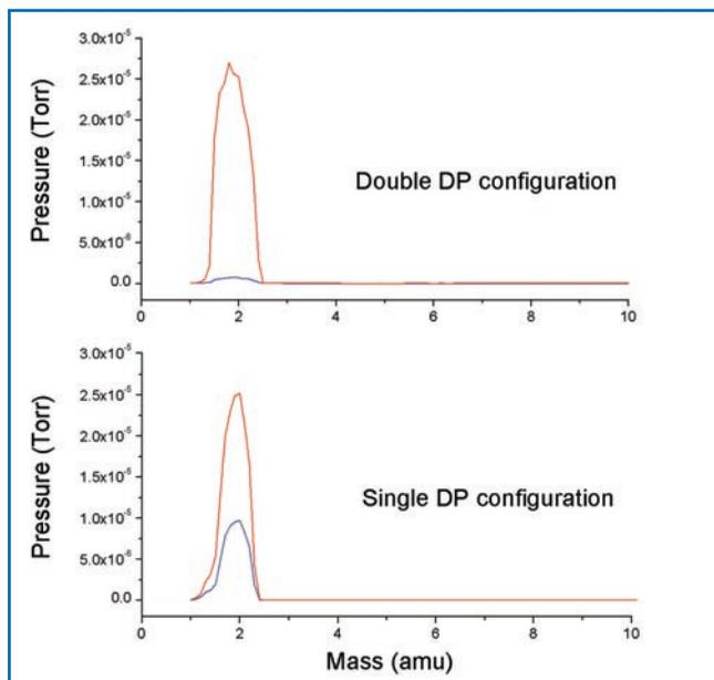
**Figure 2.** Results of the H<sub>2</sub> measurements from two different configurations; Single DP and Double DP. The red traces indicate the detector response with the sample valve open, while the blue traces show the response with the valve closed.
