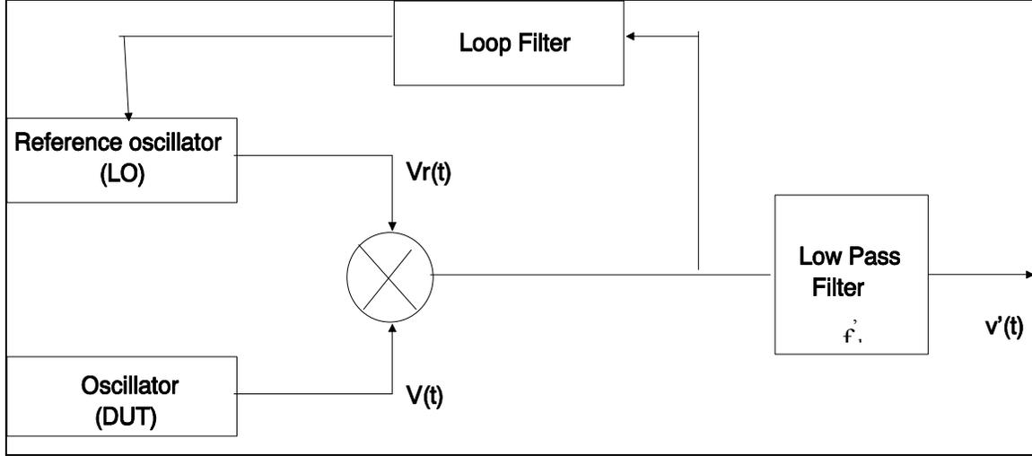
Phase noise measurements are done by mixing the device under test with a very low phase noise reference oscillator which is “loosely” phase locked at  $90^\circ$  to the device under test. Let the “ideal” reference be
