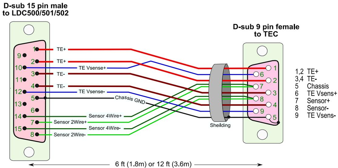
Figure 3 - TEC cable with mating connector. SRS part number O500C4 (6 ft) or O500C6 (12 ft)
