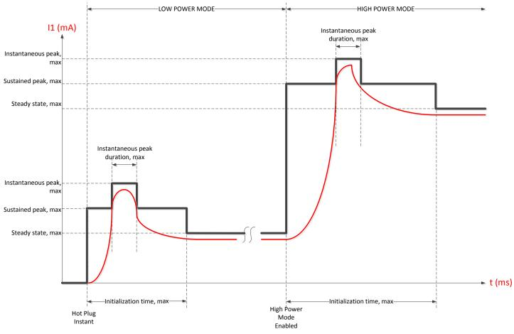
FIGURE 5-5 QSFP28 INRUSH CURRENT TIMING
