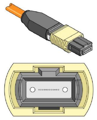
FIGURE 6-4 MPO OPTICAL PATCH CORD
