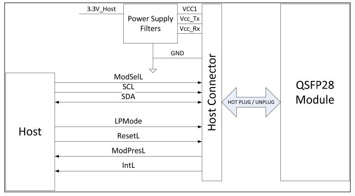
FIGURE 8-1 BLOCK DIAGRAM OF MODULE CONTROL SIGNALS
