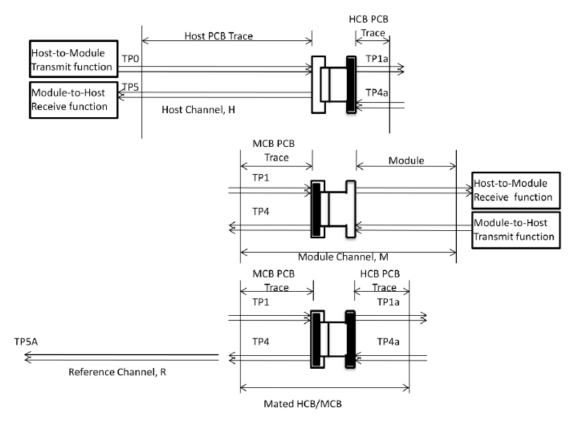
FIGURE 4-1 REFERENCE POINTS AND COMPLIANCE BOARDS
