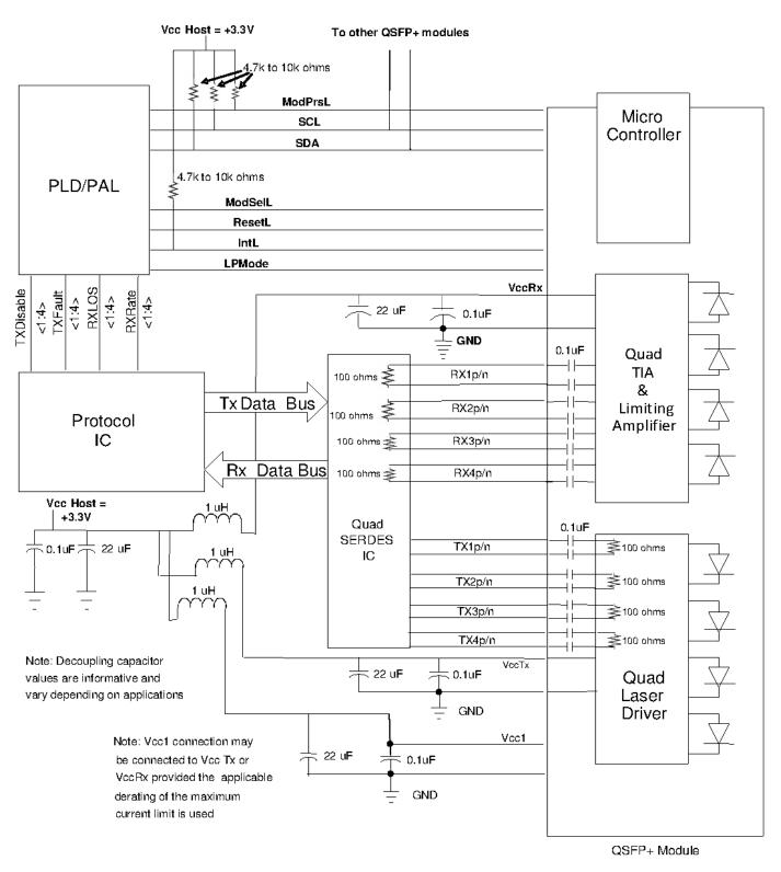
FIGURE 5-2 EXAMPLE: HOST BOARD SCHEMATIC FOR OPTICAL MODULES
