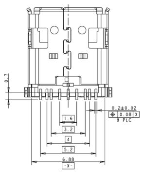
FIGURE 4-2 RECEPTACLE DIMENSIONS (2 OF 2)
