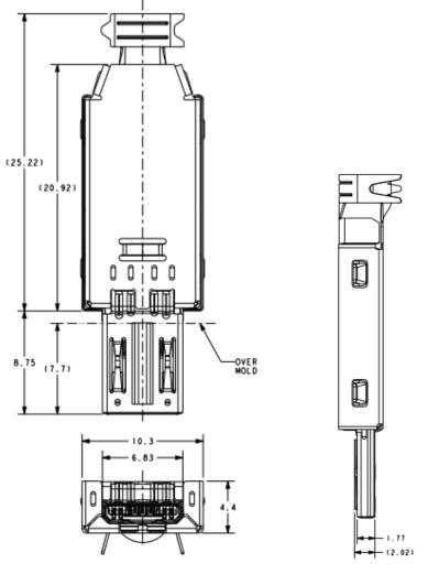
FIGURE 4-6 PLUG SHELL DIMENSIONS
