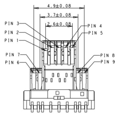
BOTTOM VIEW WITHOUT SHELL FIGURE 4-3 RECEPTACLE INTERFACE DIMENSIONS
