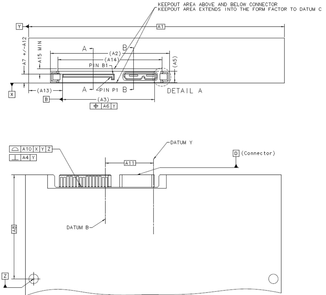
FIGURE 17-1 OPTION 1: CONNECTOR REFERENCED TO BOTTOM MOUNTING SCREWS (1 OF 2)
