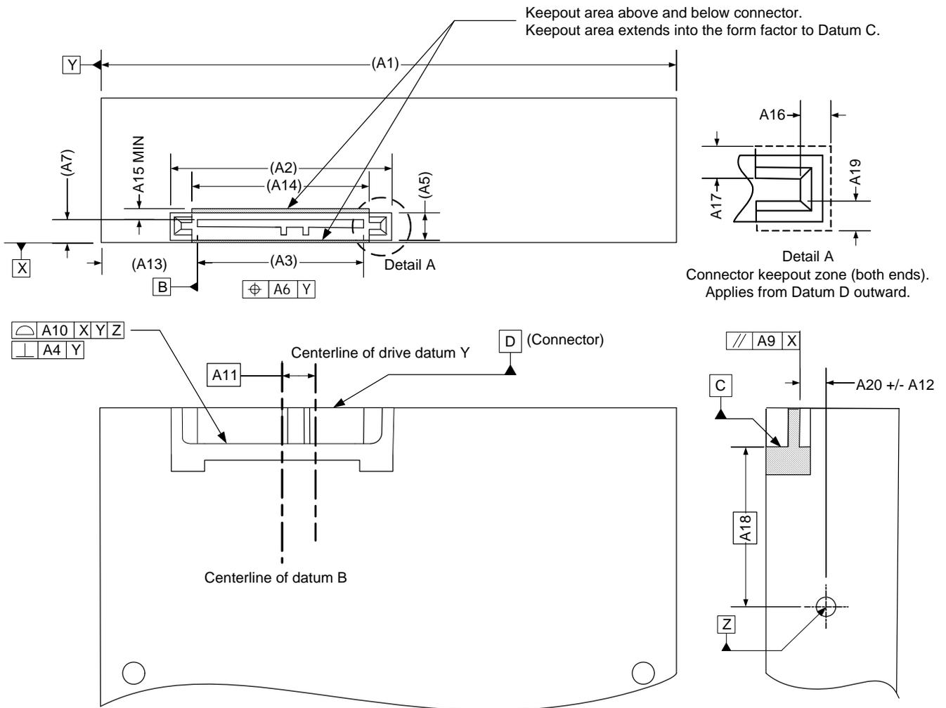
FIGURE 11-2 OPTION B: SERIAL CONNECTOR REFERENCED TO SIDE MOUNTING SCREW
