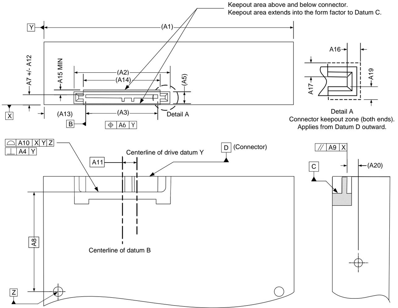
FIGURE 11-1 OPTION A: SERIAL CONNECTOR REFERENCED TO BOTTOM MOUNTING SCREW
