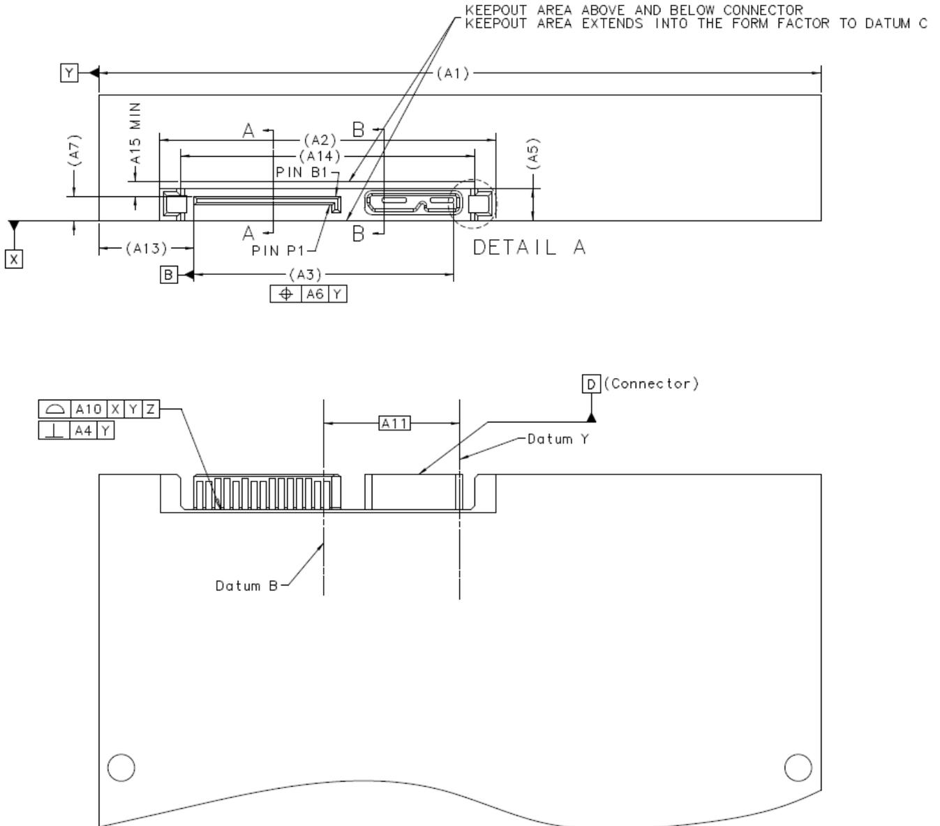
FIGURE 17-3 CONNECTOR REFERENCED TO SIDE MOUNTING SCREWS (1 OF 2)
