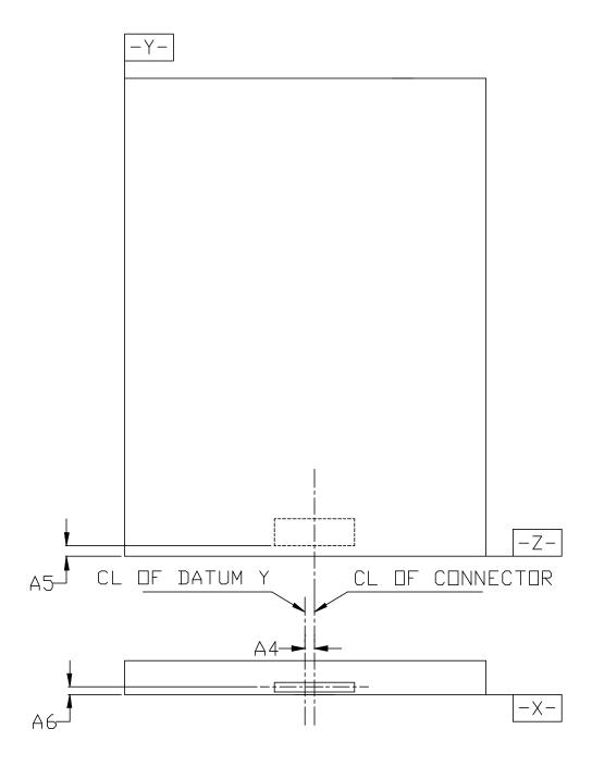
Figure 1: CE-ATA x4 and x8 Connector Position in the 54x71mm Form Factor Drawing
