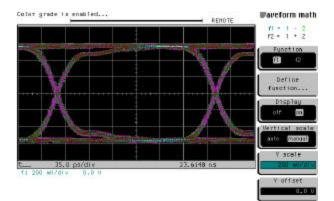
Reference Trace (No SCA-2 Connectors) 4.25 Gbps, 2<sup>7</sup>-1 PRBS 1000mV, 9 ps jitter Vertical Receptacle-Straddle Mt. Plug 0.94V, 11 ps jitter
