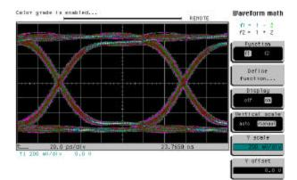
Reference Trace (No SCA-2 Connectors) 8.5 Gbps, 2<sup>7</sup>-1 PRBS 1000mV, 9 ps jitter Vertical Receptacle-Straddle Mt. Plug 0.94V, 9 ps jitter
