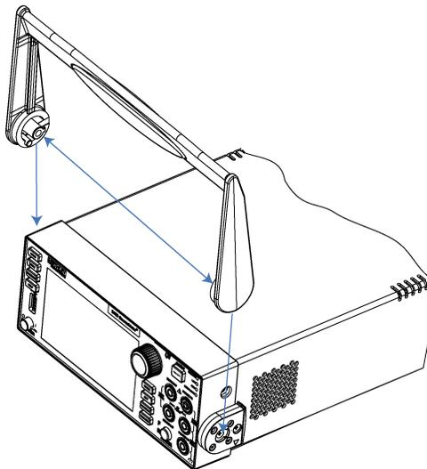
2. Align the raised flanges in the handle with the large holes in the handle-mount assembly and release the ends of the handle.
