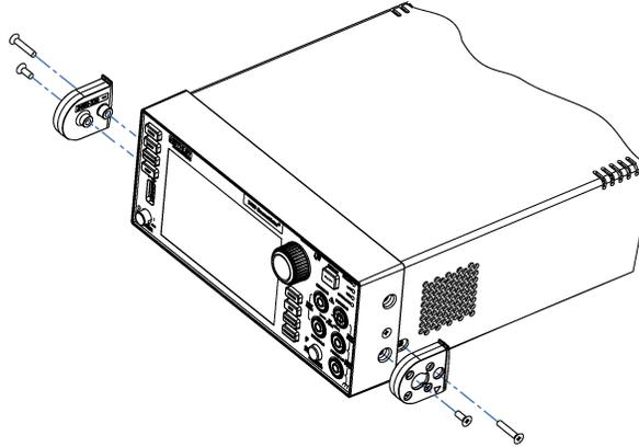
3. Insert one of the 6-32  $\times$  3/4 screws through the handle-mount assembly into the mounting hole that is closer to the rear of the instrument. Tighten using a Phillips screwdriver.
