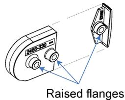
2. Align the handle-mount and cap assembly with the two lower mounting holes on one side of the instrument. Ensure that the flat edge of the assembly is facing the rear of the instrument and the raised flanges are placed inside the mounting holes.
