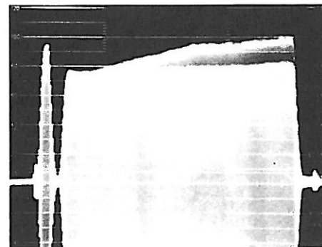
Figure 5. Difference in differential gain between two adjacent video heads as observed on a 1480-Series Waveform Monitor.
