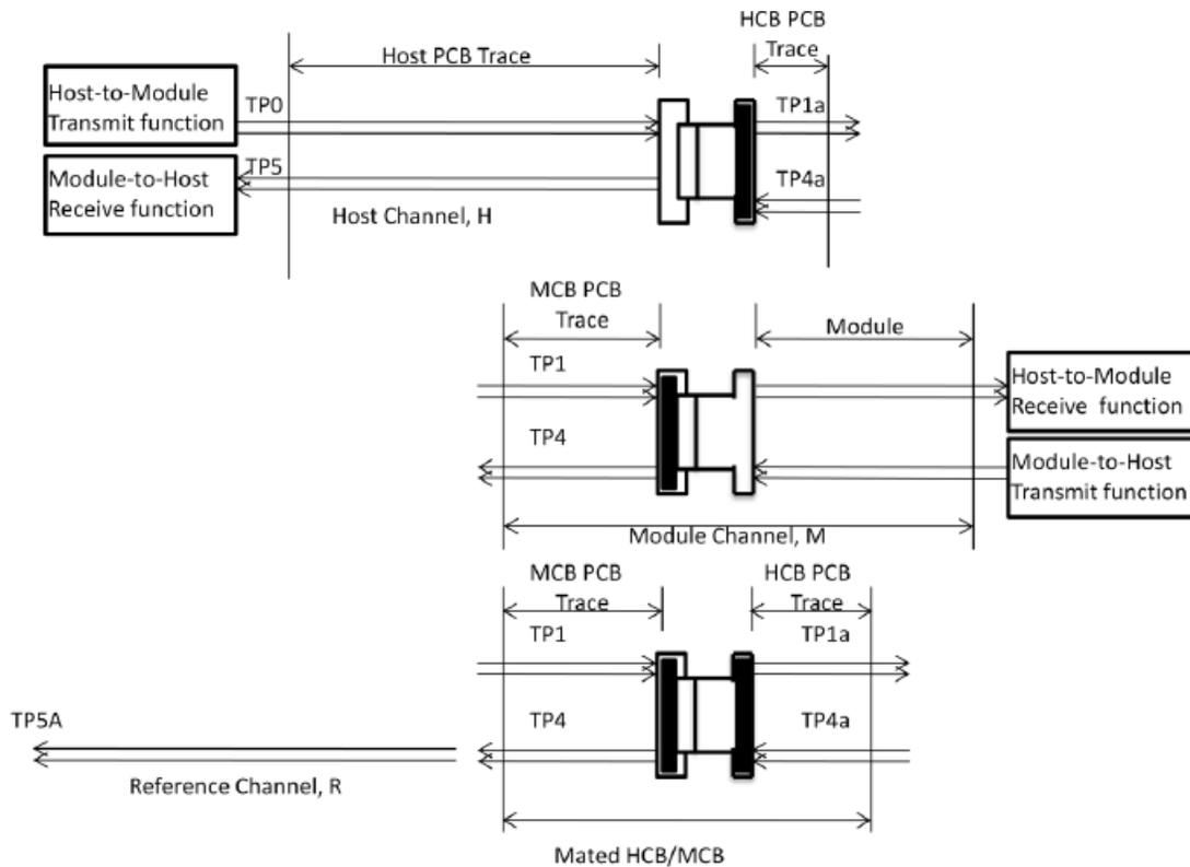
FIGURE 4-1 REFERENCE POINTS AND COMPLIANCE BOARDS
