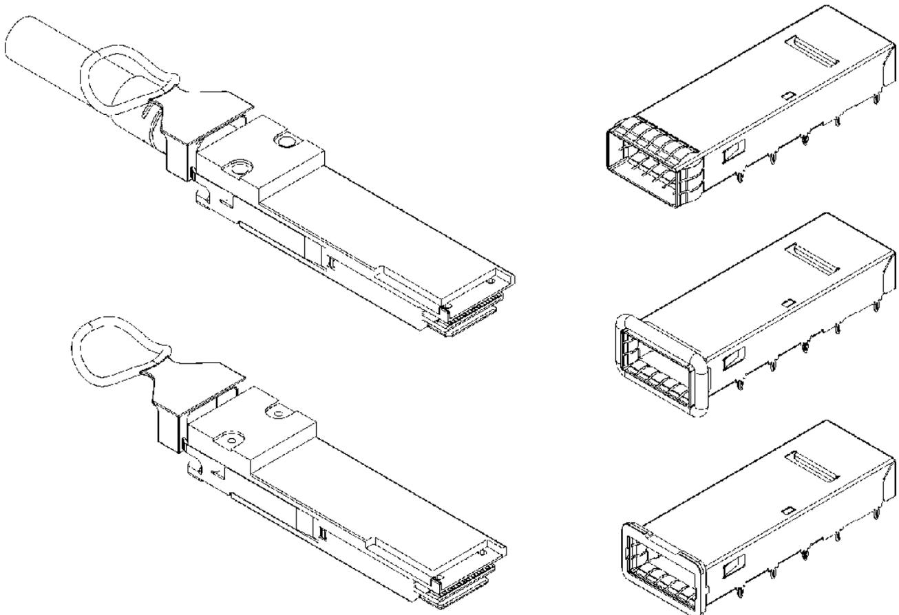
**FIGURE 6-1 PLUGGABLE AND DIRECT ATTACH MODULE RENDERING**
