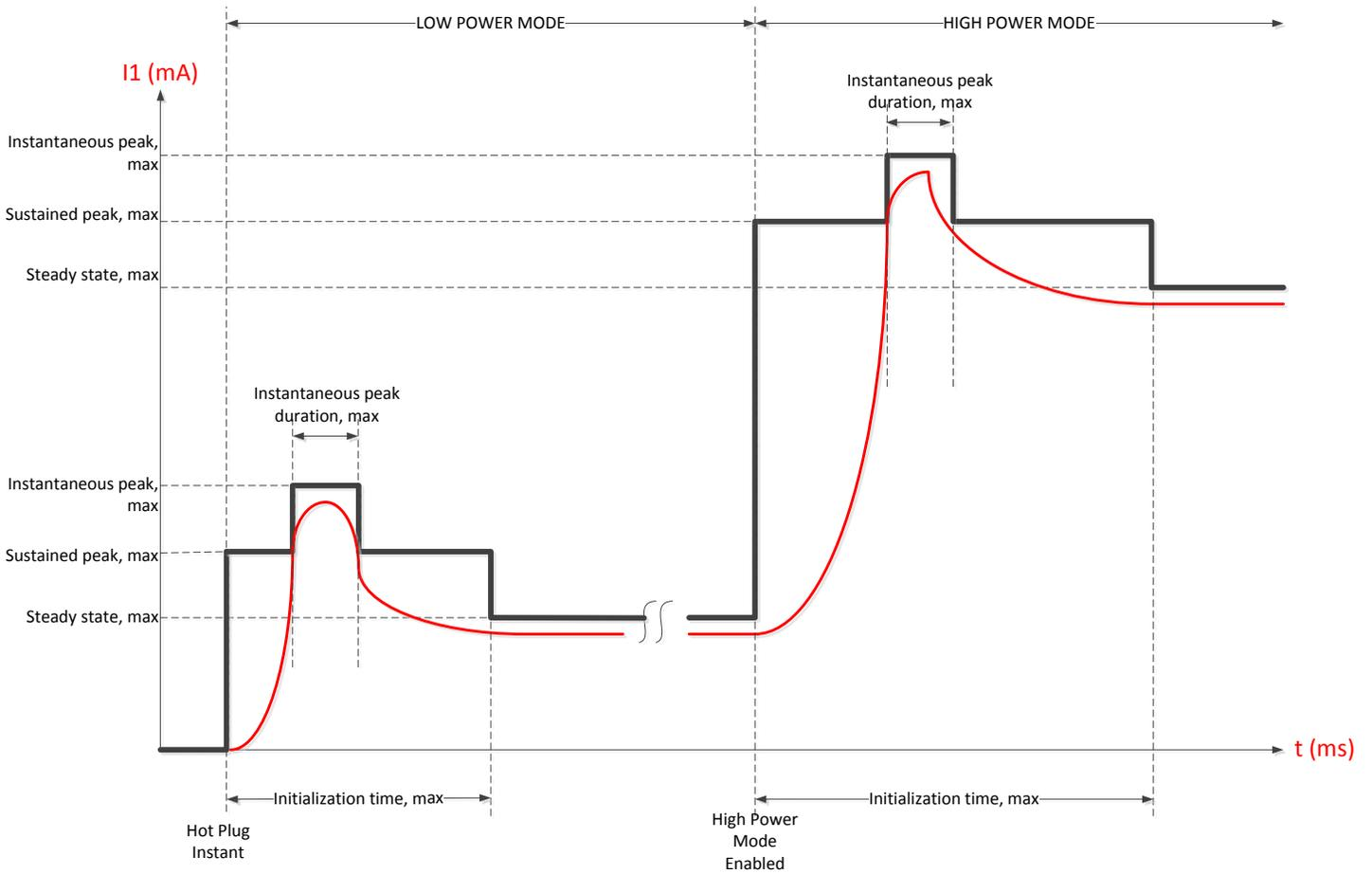
FIGURE 5-5 QSFP28 INRUSH CURRENT TIMING
