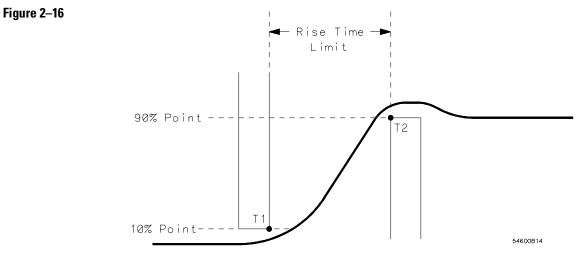
Example of a definition of a rise time testing mask
