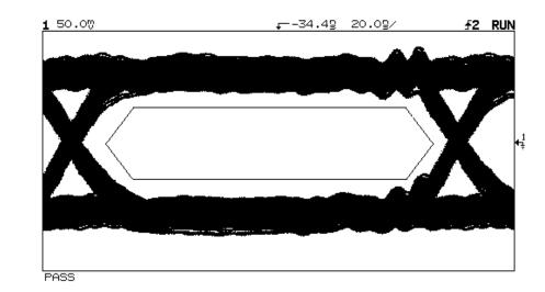
Example of a mask template used for eye-opening testing
