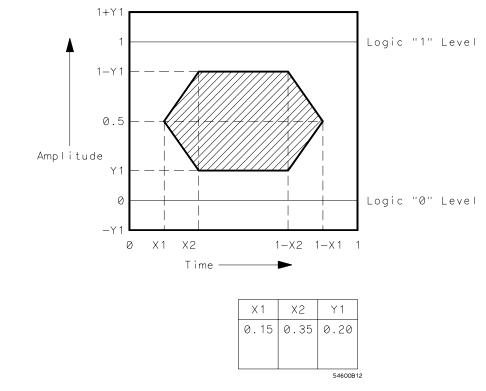
Example of the definition of an eye-pattern testing mask
