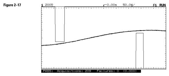
Example of a mask template for testing rise time
