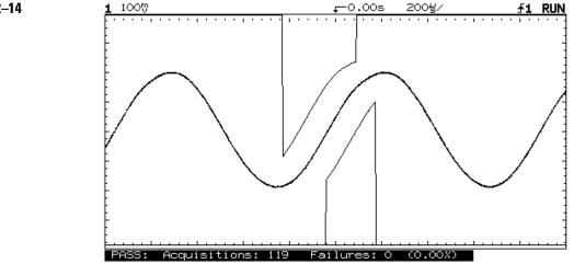
Example mask for testing the frequency of a sine wave
