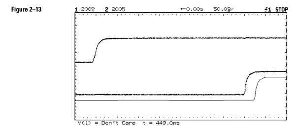
Example of a mask template used in channel to channel delay
