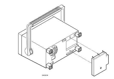
Installing the Measurement/Storage Module
