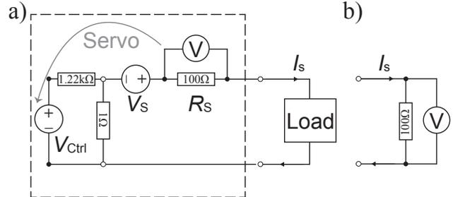
Fig. 1. The schematic of the current source and a possible scheme for the current measurements. (a) The main circuit with a voltage compensation function to stabilize the current. The feedback is represented by the grey line. (b) Current measurement based on an external  $100 \Omega$  resistor and a voltmeter.
