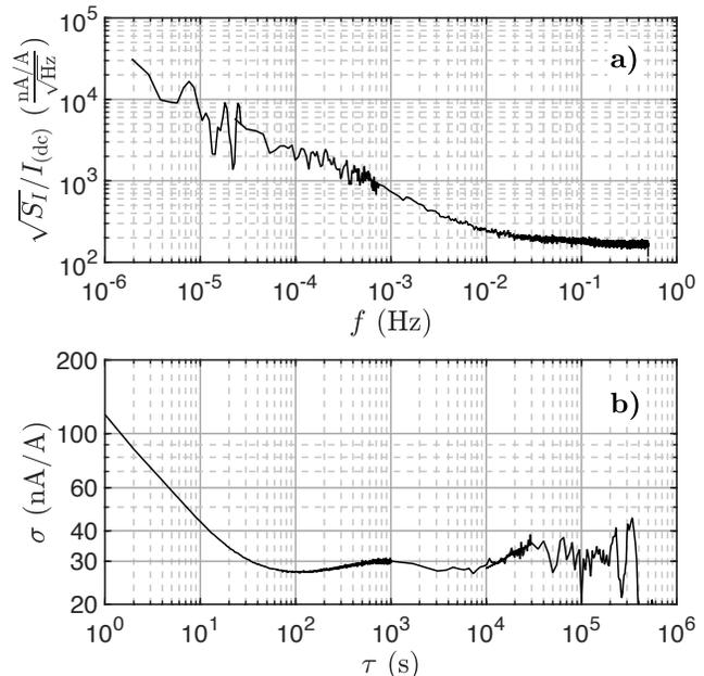
Fig. 2. (a) Noise spectrum and (b) Allan deviation of a 48 mA current measured by a LTZ1000 referenced voltmeter. The white noise density is determined to be 8.2 nA/ $\sqrt{\text{Hz}}$ . The stability is a few parts in  $10^8$ .
