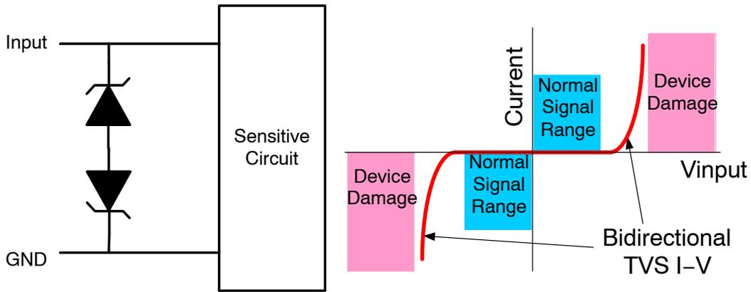
Figure 4. Application of a Bidirectional TVS Device
