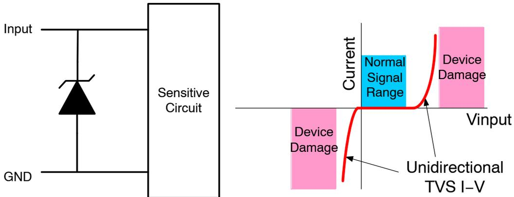
Figure 2. Application of a Unidirectional TVS Device
