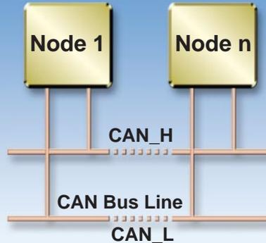
Evaluating the physical layer in the Controller Area Network (CAN) bus widely used for automotive applications is essential to analyzing communication failures that may occur, in particular, for such reasons as noise resulting from surge voltages or level fluctuations resulting from post-wiring overloads. The CAN BUS SIGNAL ANALYZER captures and analyzes the waveforms of bus signals that proved difficult with conventional protocol analyzers alone.
