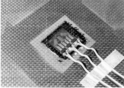
Following are some supplementary techniques for producing a chemically clean, dull matte finish needed for making good strain gage installations on these materials.
