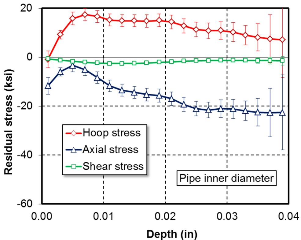
Figure 2: Residual stress measurement data from hole drilling at the inner diameter of a welded pipe
