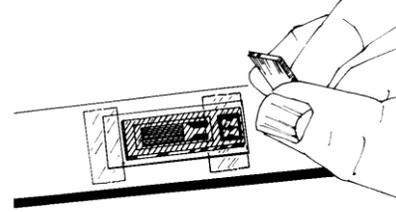
Return gage/terminal assembly to its original position over layout marks. Use only enough pressure to allow assembly to be tacked down. Overlay gage/terminal area with a piece of thin TFE-1 teflon film. If necessary, anchor Teflon in position with a piece of mylar tape across one end.
