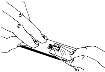
The gage and terminal strip are now solidly bonded in place. To remove the tape, pull it back directly over itself, peeling it slowly and steadily off the surfaces.
