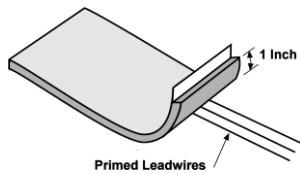
Cut a patch of M-Coat FB butyl rubber sealant large enough to extend 1/2 in [13 mm] beyond the three open sides of the gage (or Teflon tape), and at least 1-1/4 in [30 mm] beyond the end of the gage or terminal strip from which the leadwires exit. If the gage-bonding adhesive extends beyond this area, increase the size of the patch accordingly. This is particularly important with M-Bond 200 cyanoacrylate adhesive.
