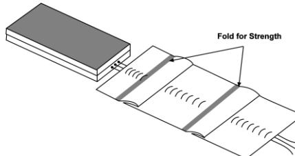
M-Coat FA aluminum tape can serve as a convenient leadwire restraint. For maximum strength, fold as shown above.
