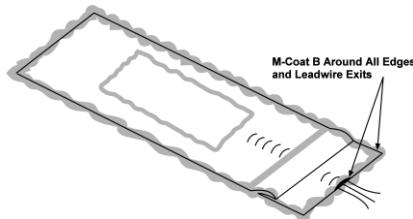
Apply two coats of M-Coat B to the tape edges paying particular attention to the lead exit area. Allow the first coat to dry to the touch before applying the second. A completed installation is shown above.
