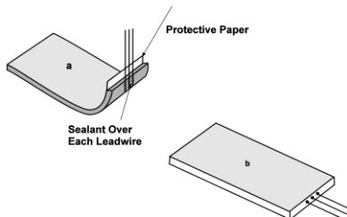
Using tweezers, raise each lead and tack to the coating. Use a dental probe to form the sealant around each lead, being careful not to puncture the sealant. Firmly press the remainder of the patch onto the specimen surface.
