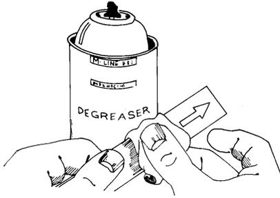
Thoroughly degrease the gaging area with solvent, such as CSM Degreaser or GC-6 Isopropyl Alcohol. The former is preferred, but there are some materials (e.g., titanium and many plastics) that react with CSM. In these cases, GC-6 Isopropyl Alcohol should be considered. All degreasing should be done with uncontaminated solvents—thus the use of “one-way” containers, such as aerosol cans, is highly advisable.
