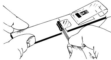
Apply a thin layer of adhesive to the gage bonding side and to the specimen. The adhesive film should be just thick enough to cover the gaging area without bubbles or voids. Approximately 0.002 in [0.08 mm] is typical on metal surfaces. Any lumps of unmixed adhesive should be removed before proceeding.
