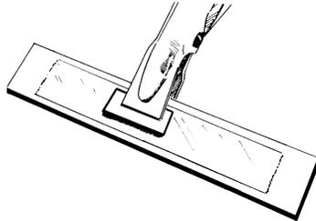
Either HSC-X spring clamps, as in, or deadweight can be used to apply pressure during the curing cycle. A clamping pressure of 10 to 30 psi [70 to 200 kN/m<sup>2</sup>] is recommended. Place clamped gage/specimen into a cool oven and raise temperature to the desired curing level at a rate of 5° to 20°F [3° to 11°C] per minute.
