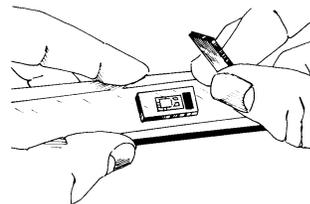
Overlay the gage/terminal area with a piece of thin Teflon sheet (TFE-1). If necessary, anchor the Teflon in position with a piece of Mylar tape across one end.
