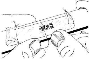
Remove the gage/tape/terminal assembly by peeling tape at a shallow angle (about 45°) and transferring it onto the specimen. Make sure gage alignment marks coincide with specimen layout lines. If misalignment does occur, lift end of tape at a shallow angle until assembly is free. Realign and replace. Use of a pair of tweezers often facilitates this handling.
