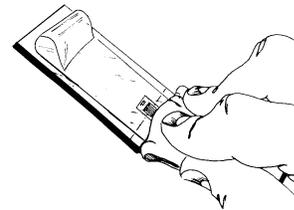
Replace the gage/tape assembly over the alignment marks on the specimen and, using a piece of gauze, slowly make a single wiping stroke over the assembly.
