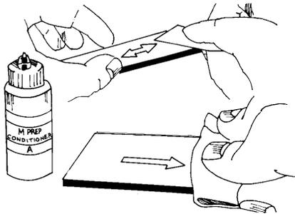
Preliminary dry abrading with 220- or 320-grit silicon-carbide paper is generally required if there is any surface scale or oxide. Final abrading is done by using 320- or 400-grit silicon-carbide paper on surfaces thoroughly wetted with Conditioner A; this is followed by wiping dry with a gauze sponge.
