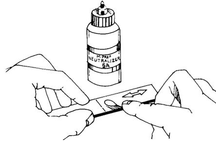
Now apply a liberal amount of Neutralizer 5A and scrub with a cotton-tipped applicator. With a single, slow wiping motion of a gauze sponge, carefully dry this surface. Do not wipe back and forth because this may allow contaminants to be redeposited on the cleaned surface.
