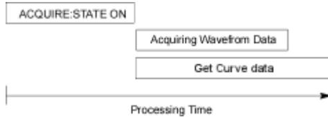
To ensure that the instrument completes waveform acquisition before attempting to execute the CURVE? query, you can synchronize the program. The figure below shows the desired processing sequence.
