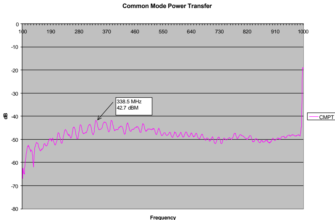
Figure 35 - CMPT calculated using Pin and Pout in Figure 34
