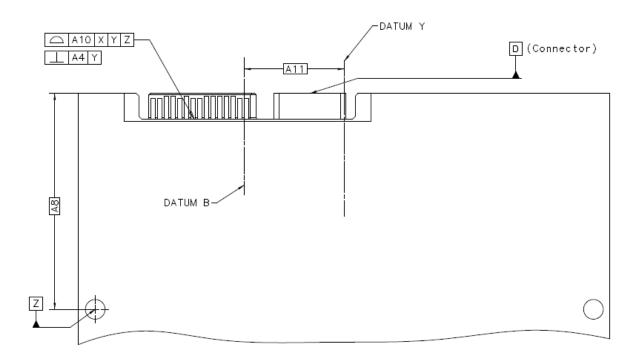
FIGURE 17-1 OPTION 1: CONNECTOR REFERENCED TO BOTTOM MOUNTING SCREWS (1 OF 2)
