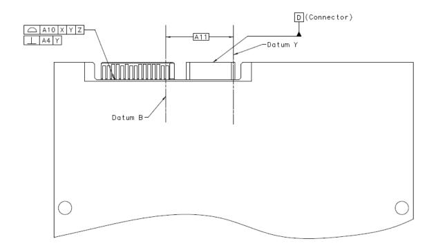
FIGURE 17-3 CONNECTOR REFERENCED TO SIDE MOUNTING SCREWS (1 OF 2)
