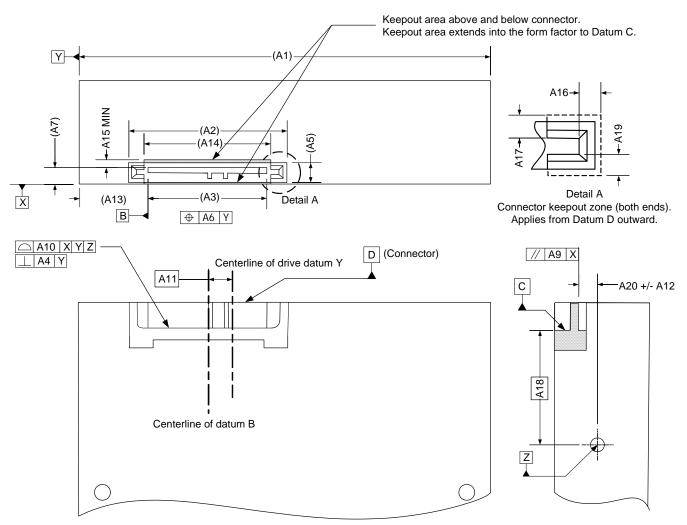
FIGURE 11-2 OPTION B: SERIAL CONNECTOR REFERENCED TO SIDE MOUNTING SCREW
