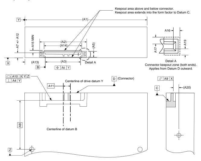
FIGURE 11-1 OPTION A: SERIAL CONNECTOR REFERENCED TO BOTTOM MOUNTING SCREW
