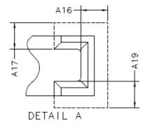
CONNECTOR KEEPOUT ZONE (BOTH ENDS) APPLIES FROM DATUM D OUTWARD
