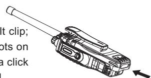
Press and hold the top of the belt clip; match the battery with the two slots on the radio and push forward until a click is heard. Then the battery is fixed.
