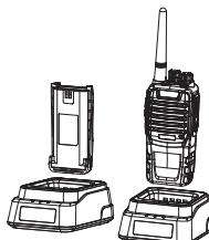
Plug the battery or radio into the charger slot, and make sure the radio has been turned off.
