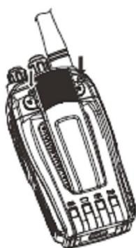
When installing, match the two screw holes to the holes on the back of the radio, use screw to fasten it; when removing, use screwdriver to remove these two screws, take off the belt clip.
