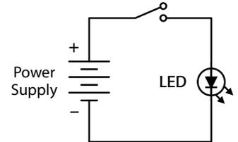
As soon as the switch closes, the charge stored at the output of the power supply and the wires flows rapidly into the LED until the power supply starts to regulate. The transient current peak is shown by the blue line in the oscilloscope view in **Figure 2 (a)**.
