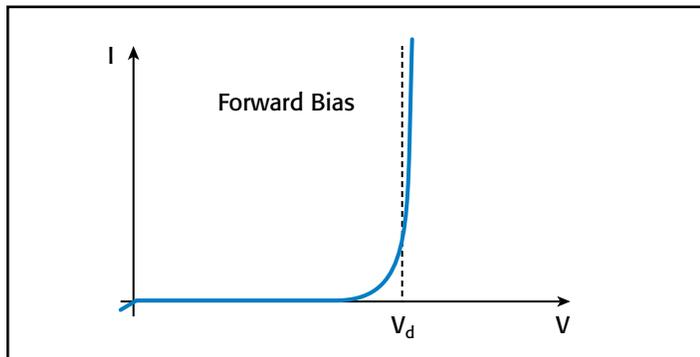
**Figure 1. Typical I-V curve of a diode.**
