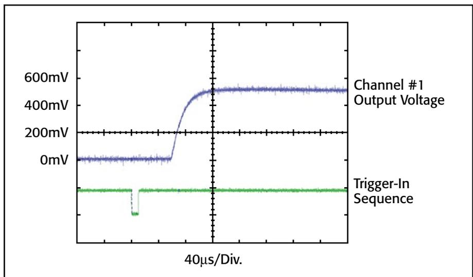
**Figure 2.** This magnified view of the first 500mV voltage step from the signal shown in Figure 1 illustrates how the Channel #1 output reaches the voltage setpoint within 160µs of the trigger-in pulse.
