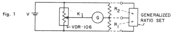
The ratio  $\rho \left( = \frac{R_1}{R_1 + R_2} \right)$  is given, at null, by the expression
