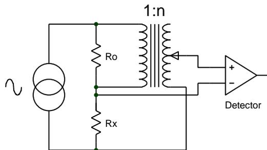
**Figure 2: AC ratio transformer bridge.**
