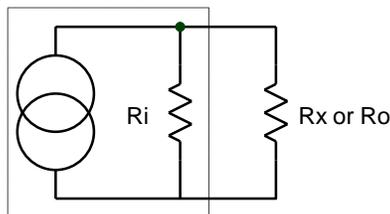
Figure 5: Effect of current source output impedance.
