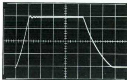
Fig. 4. Response at 411A output terminal to a full-scale burst of rf applied to 411A input. Sweep time is  $\frac{1}{2}$  sec/cm; vertical scale is  $\frac{1}{2}$ -volt/cm.
