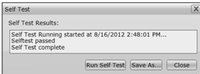
**CAUTION** If the Self Test fails, it indicates which module is likely to need service. See "M9380A Troubleshooting" on page 33 to ascertain the source of the failure.
