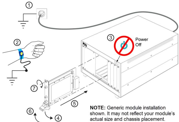
7. Secure all modules to the chassis using the module mounting screws. Use a #1 Pozidriv® or a slotted screwdriver and torque to 5 Lb-In (0.57 N-m). Performance may suffer if the screws are not tightened properly.
