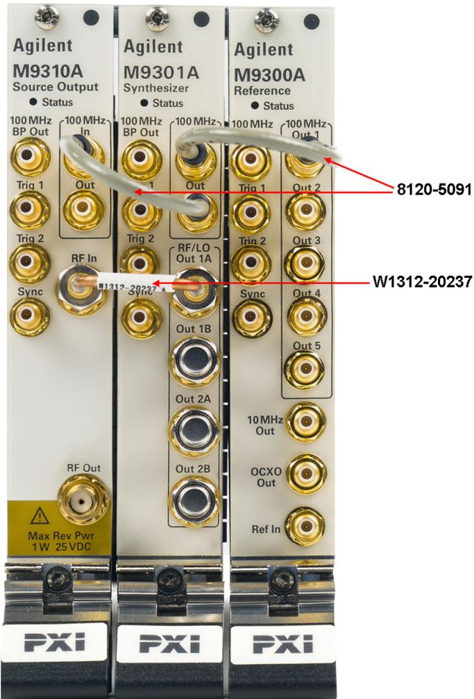
**Recommendation:** Install the semi-rigid cable first.
