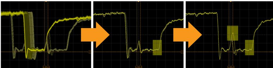
With the InfiniiScan Zone touch trigger, if you can see it, you can trigger on it.
