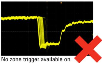
No zone trigger available on the Tektronix 4000B.
