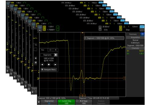
Optimized and efficient segmented memory architecture in the 4000 X-Series selectively captures critical signal details over 66 seconds at 5 Gsa/s. It not only captures 1,000 metastable signals, but reveals critical delta time relationships among them.
