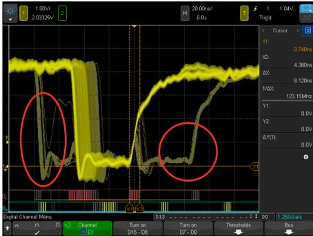
Both analog and digital channels are turned on. Many infrequent glitches and metastable signals were observed after 10 second of acquisition on the 4000 X-Series.
