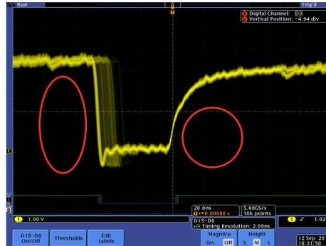
Both analog and digital channels are turned on. Even after 60 seconds of acquisition, Tektronix 4000B failed to capture any glitches or metastable signals.
