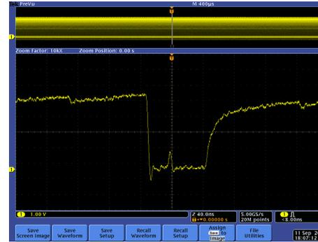
At 5 GS/s and 20 Mpts, a traditional memory architecture scope like the Tektronix 4000B can only capture 4 ms of signals. This may be able to capture 1 glitch, but certainly not to analyze inter-glitch timing correlations which are multi-milliseconds apart.
