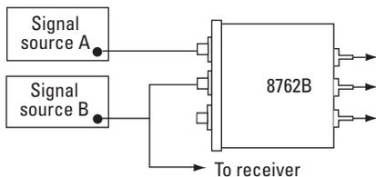
Figure 4. Multi-source switching
