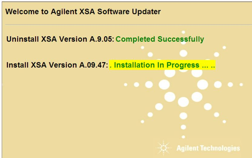
The new instrument software is being installed. The “Installation in Progress” text will roll across the screen indicating software activity. There will be several windows appearing and disappearing during this time. NO interaction with the instrument is required. Please be patient the total software installation process can take 30 to 40 minutes. It will display “Completed Successfully” when the software update is complete. You will be prompted to restart you instrument at the end.
