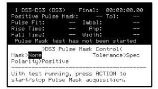
Press ACTION to begin the pulse mask test.
