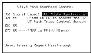
VT Path Overhead Bytes: Each byte can be set as described below.
