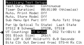
**VT Counting Mode** sets the method for specifying VT channels. This parameter can be set as follows:
