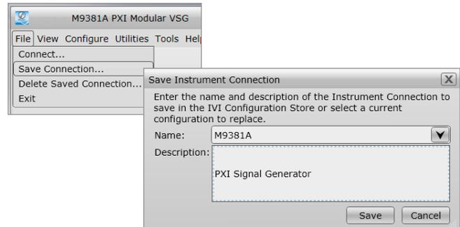
Figure 7. M9381A soft front panel saving connection name.
