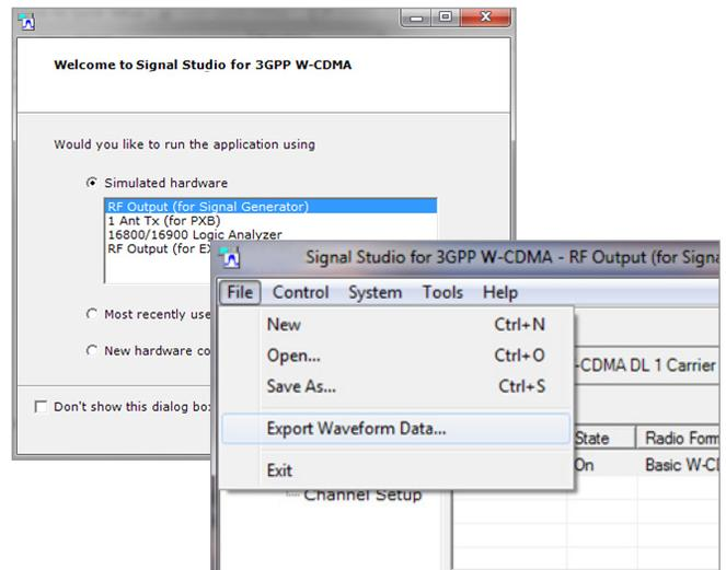
Figure 9. Saving a waveform file from Signal Studio.
