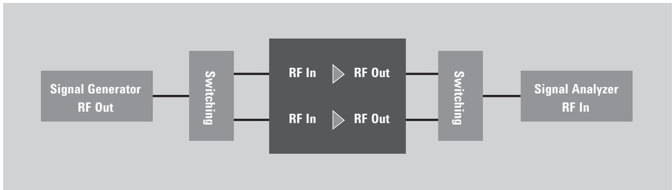
Figure 2. Typical Power Amplifier/Front End Module Test Setup.
