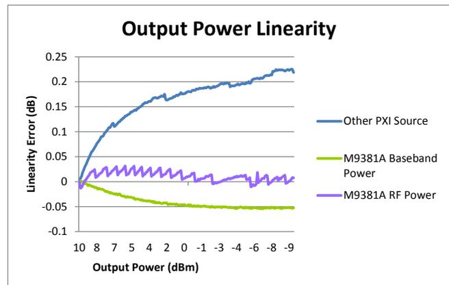
Figure 3. Note M9381A linearity error within  $\pm 0.05$  dBm range.
