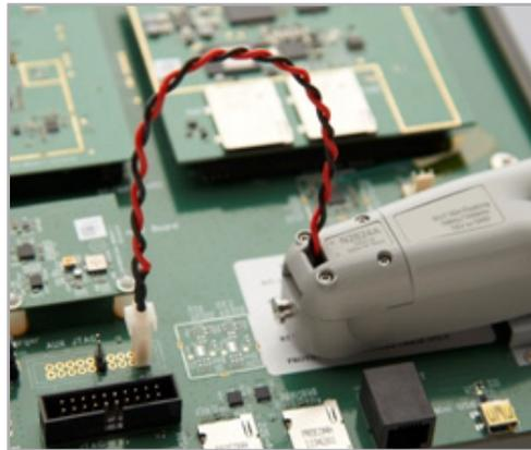
Figure 4-4. The supplied Make-Before-Break (MBB) connectors allow you to quickly probe multiple locations on your DUT without having to solder or unsolder the leads.
