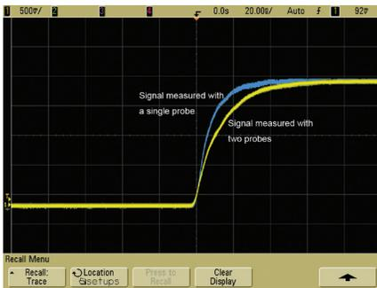
Fig 2-1. Probe loading check with two probes
