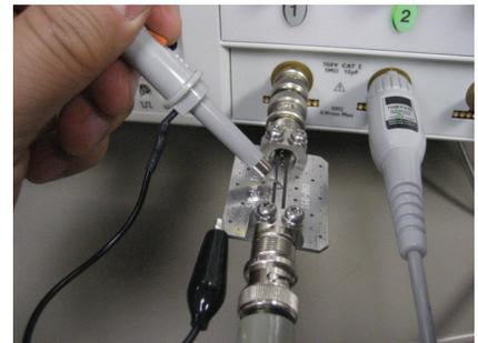
Figure 2-2. Probe loading caused by a long ground lead
