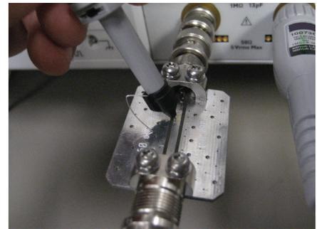
Figure 2-3. Reduced probe loading with short ground lead
