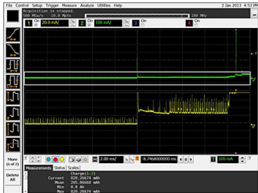
Figure 4-5. Keysight's Infiniium and InfiniiVision oscilloscopes provide an area under the curve measurement (Charge), where you can easily calculate the integrated current consumptions in Ah (Ampere x Hour) over time.
