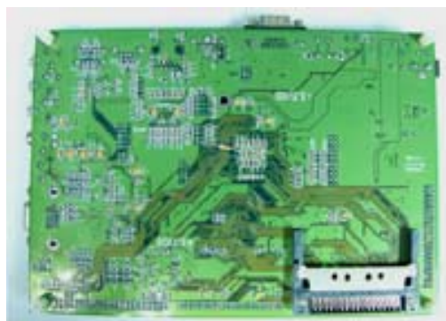
NK9312 Evaluation Board with EP9315 processor and a PCMCIA interface on the rare of the board
