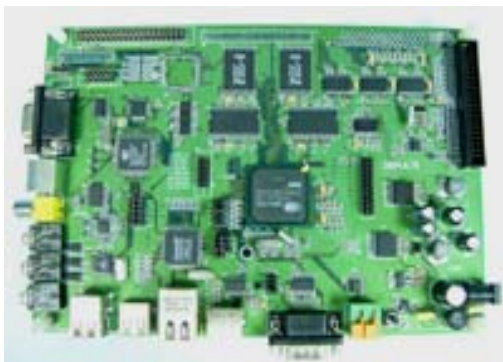
NK9312 Evaluation Board with EP9315 processor and a PCMCIA interface on the rare of the board
