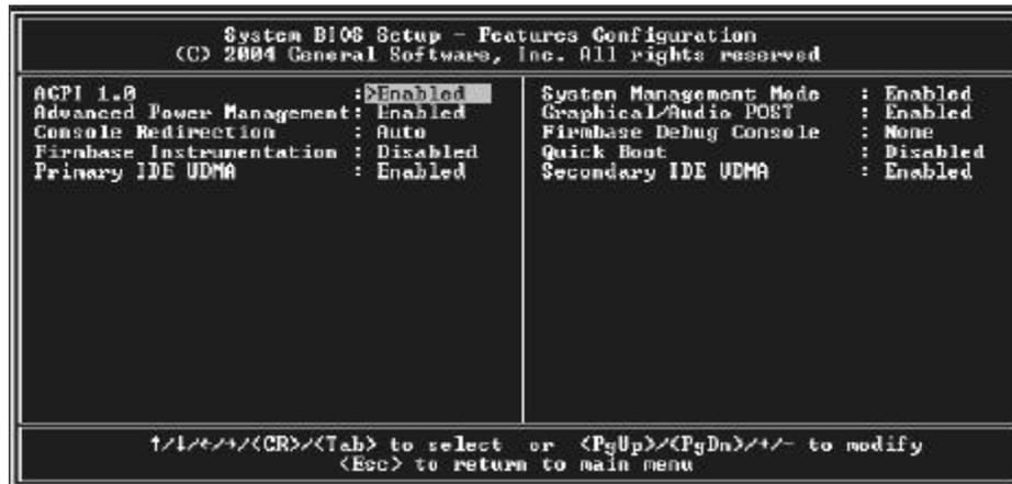
Figure 3.8. The Embedded BIOS 2000 Features Setup Screen allows you to re-configure BIOS-level features.
